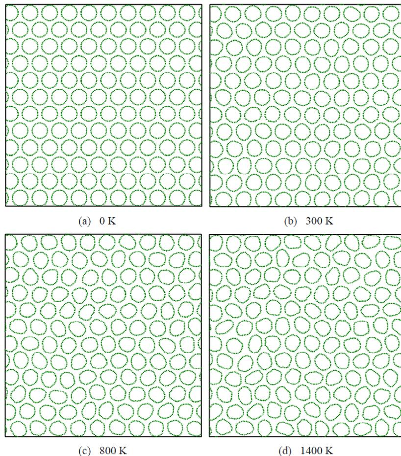
**Fig. 4.** Images of the structure of a CNT bundle at different temperatures: (a) 0 K, (b) 300 K, (c) 800 K and (d) 1400 K. The case of  $N=30$  is presented.
